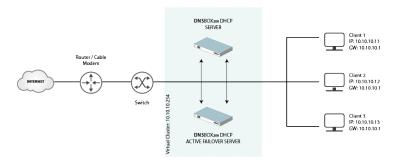
Active – Passive mode - achieved by clustering a pair of DHCP servers on a single virtual IP address. A passive server copies information about the leases distributed by the active server in real time.
